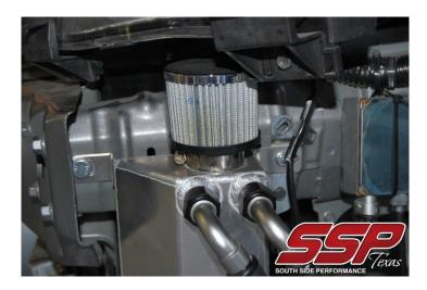
Step 4: Route hoses. There are 2 hoses, they will need to be cut to length. The first hose will go on the PCV hose routing back to the intake. You need to remove the OEM hose, attach the new hose to the valve cover. If you are still routing the oem hose back into your intake, there is a supplied red high temp cap for your intake.
