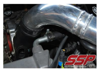
The other hose you will need to cut to length will go on the oem PCV plate. This PCV hose on the PCV plate is the same plate everyone puts a catch can on now. The catch can hose will attach to the green pcv fitting on the block. The other end on the intake manifold will be capped off with the supplied red high temp cap. You can access this from under the car however it is very tricky and easier in installation to remove the intake manifold.
