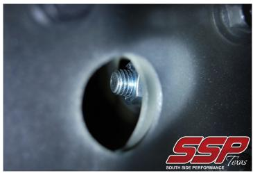
Note: Some "adjustment" may need to be made to the mounting bracket on the horn so it clears:
