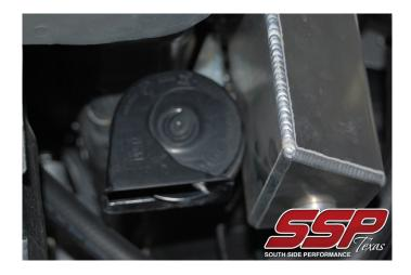
Step 3: Secure large bolt, large nut and small 10mm nut that mounts catch can.
