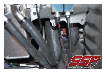
Step 5: Make sure the filter and Allen drain plug are secure on the can if not already. We recommend using thread sealant tape on the threads of the drain plug to assure no small leaks in the can.
