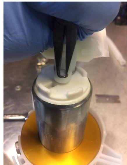
**Step 5:** Install PTFE fuel hose onto fuel pump outlet and secure with clamp. Orient the fuel line as shown in the pictures below. Click the new fuel pump assembly into the bottom basket. Install the top hat back on the basket with the C-Clip we removed earlier. Install the new PTFE fuel line onto the top hat barb and secure with clamp. Plug in electrical connections and install into car. Enjoy!
